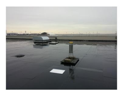
The primary area used for official snow measurements at JFK International Airport denoted by the white SMB in the photo. This is a view looking southeast. An 8-inch standard rain gauge is also located on the roof as a back-up to the ASOS at JFK.
