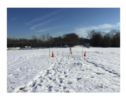
**Measurement Area** - During the blizzard, the site was located on a relatively flat grassy area, subtly higher in terrain than the surrounding area. Aside from a 7 foot tall chain link fence located about 130 feet to the northeast, the nearest wind obstruction was a 30-40 foot tall tree located approximately 170 feet to the east. Other wind breaks (trees) to the north were about 500 feet away. Exposures in other directions were virtually unlimited. The site was located about 600 feet
