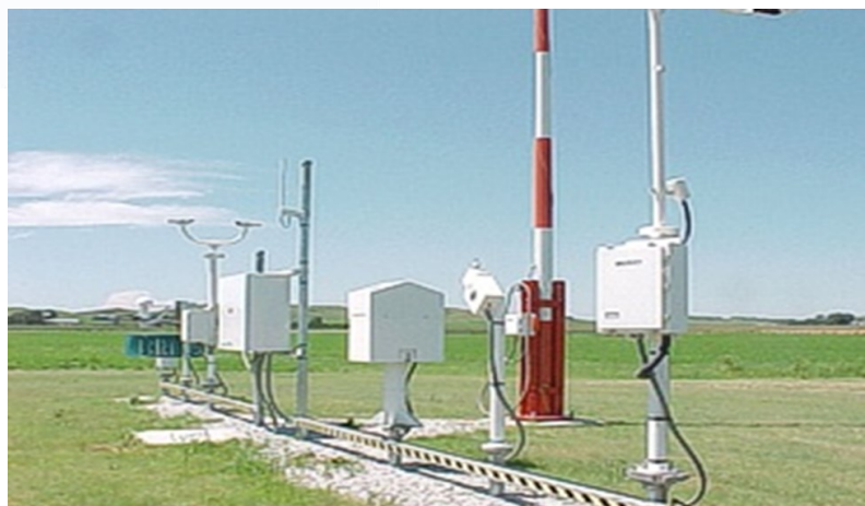
A "typical" automated airport weather system.
