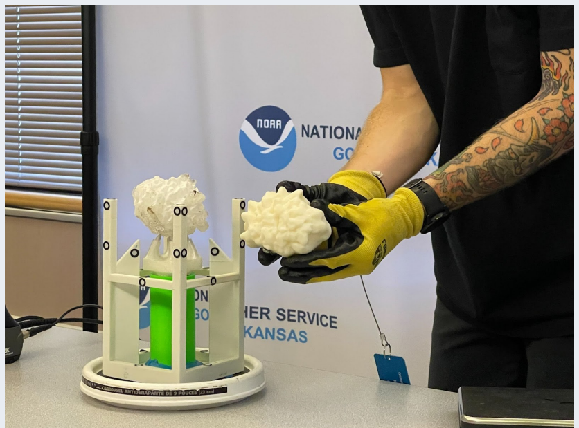
An IBHS expert measures the Kirk hailstone using a 3D laser scanner while visually comparing it to the Bethune hailstone in his hand. Image: NWS Goodland
