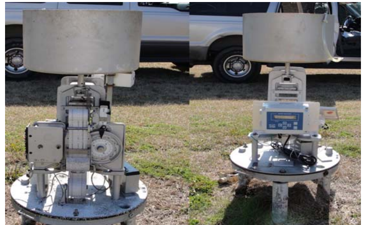
Fisher-Porter gage with punch mechanism (left) and with the new digital logger (right).
